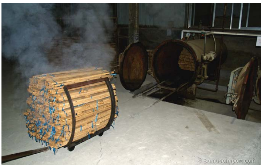
Figure 44: Boiling of bamboo strips process
