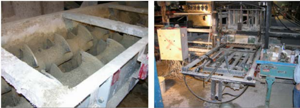
Figure 21: Device for pre-casting hempcrete blocks – mixer, forming process (Collet et al., 2013)
