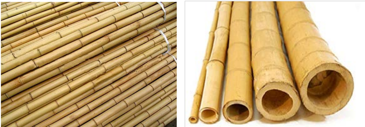
Figure 28: Bamboo poles: (a) Cured and treated poles (b) Various geometry and sizes of bamboo poles
