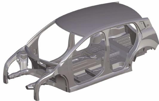
High strength steel which is used to make lighter weight automotive and EV car bodies
