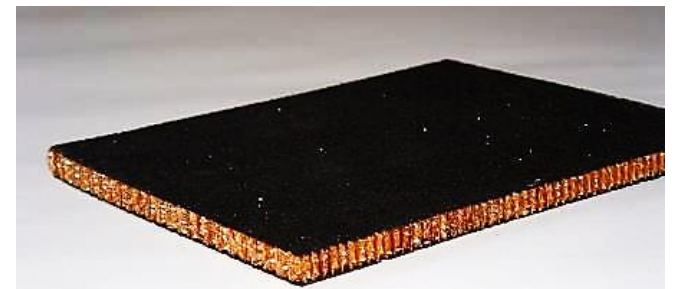
Panel from woven flax fabric and thermoset resin
