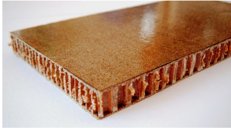
Panel from woven flax fabric thermoset resin
